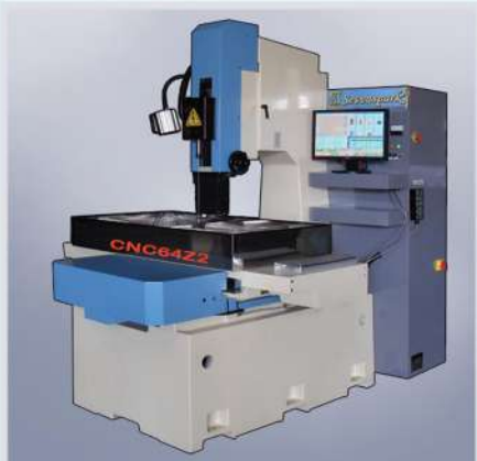
CNC on X Y Z. Drived by AC servo motor. Z2 button up down. Dialog windows editing. Portable keyboard +Hand pendant.
