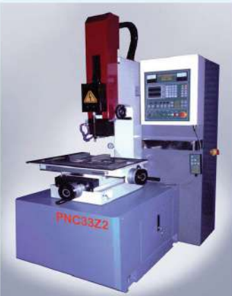
PNC35Z2 PNC43Z2 PNC54Z2 PNC64Z2 PNC75Z2 Z axis NC automated drilling. 99 sets EDM parameters inside. IO interface fit for Rotary table.
