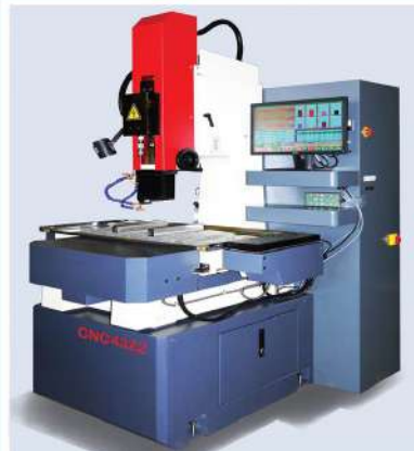
CNC on X Y Z. Drived by AC servo motor. Z2 button up down. Dialog windows editing. Portable keyboard +Hand pendant.
